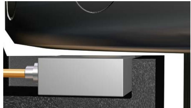
Measuring the thermal expansion
