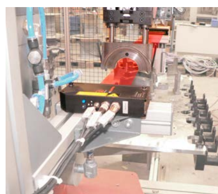
Bearing shell detection in automotive manufacturing
