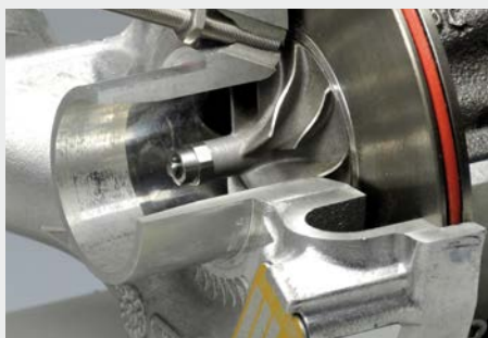
Rotational speed measurement of turbochargers
