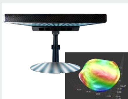
3D shape measurement of wafers
