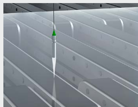
Thickness measurement of flat glass
