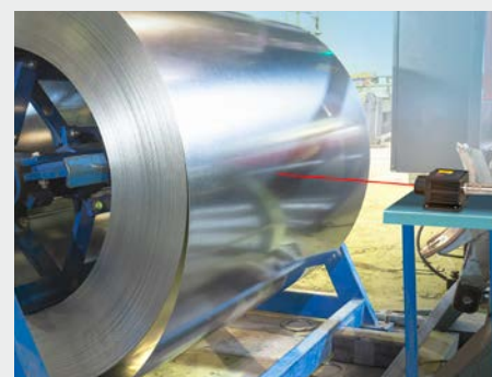
Acquisition of coil diameters
