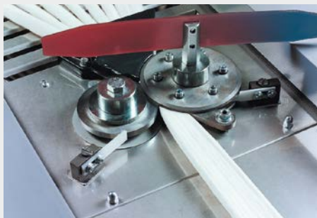
Inline yarn thickness measurement
