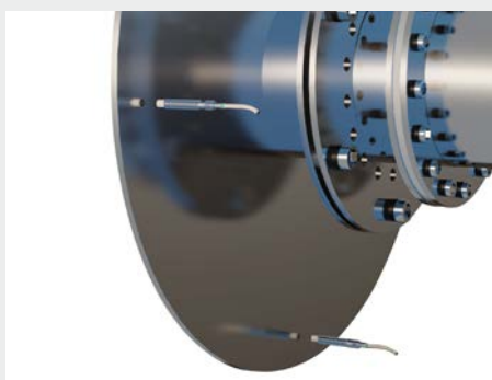
Measuring the radial runout of clutch discs
