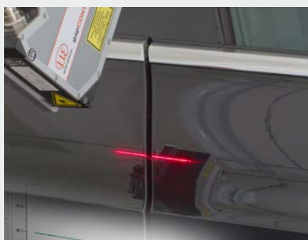
Gap and flushness measurement on bodywork parts
