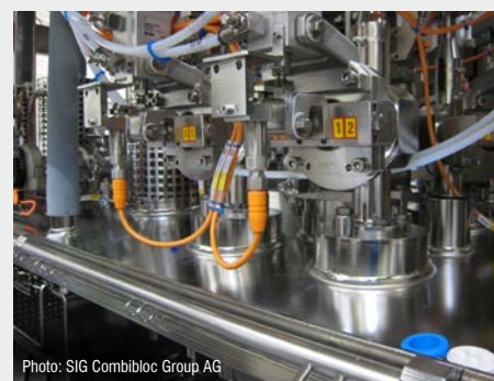
Valve lift measurement in the food industry
