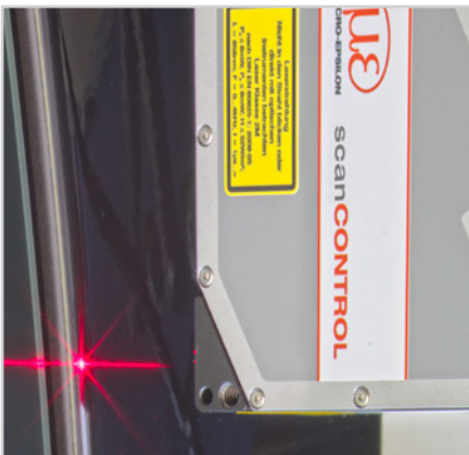
Gap measurement on car bodies
