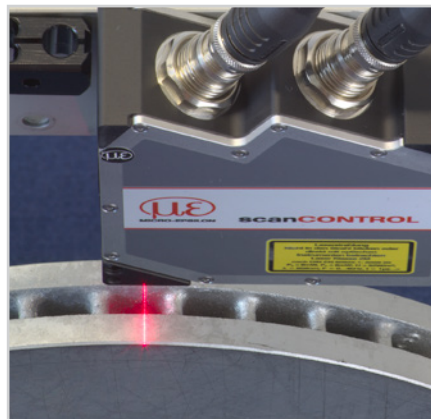
Profile measurement of the brake disc
