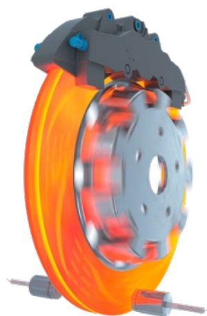
Thickness measurement of brake discs
